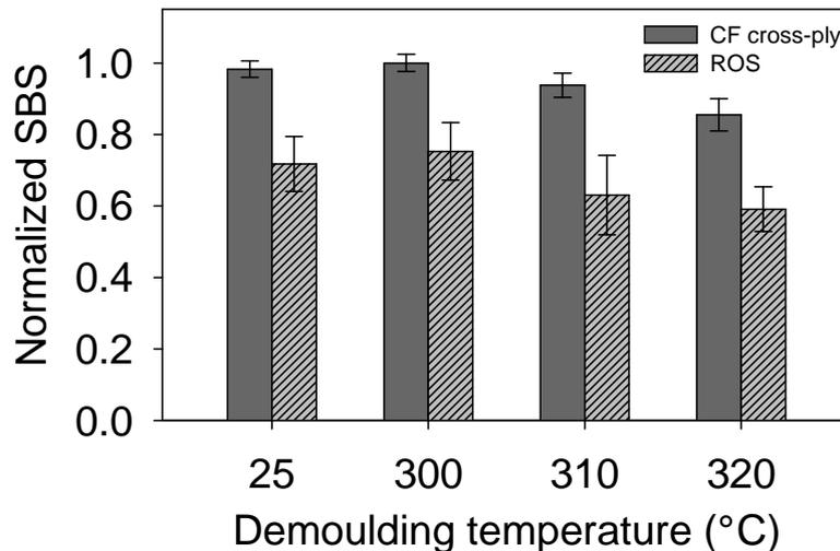
**Figure 1:** Normalized short-beam strength as a function of the demoulding temperature. The error bars show  $\pm$  one standard deviation.
